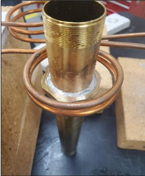
The assembly inside the four-position induction coil.
