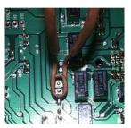
Coil in place to heat two preforms
