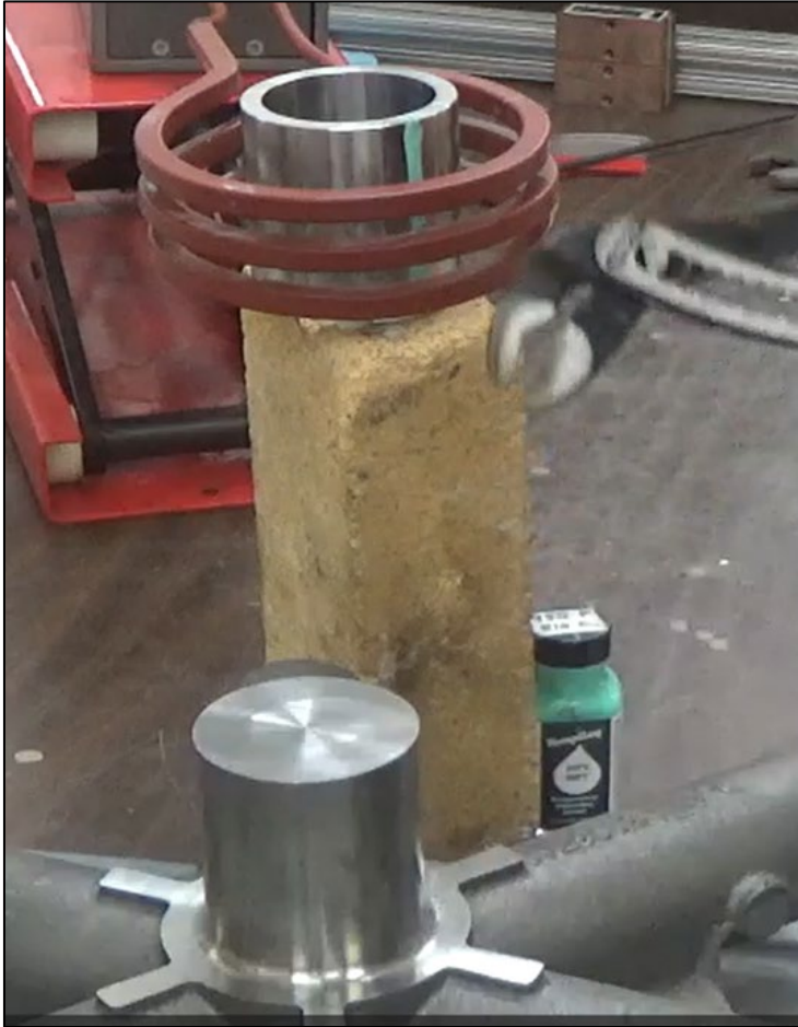
The steel sleeve assembly, with a component of it in the coil, prior to press fitting.
