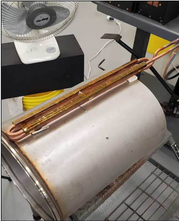
The coil over the weld seam
