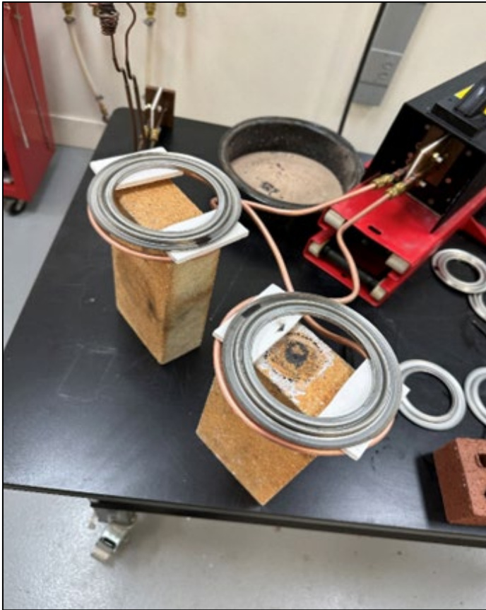
The induction setup with the pancake coil and customer-supplied parts.
