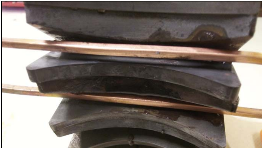
The assembly inside the induction coil prior to brazing
