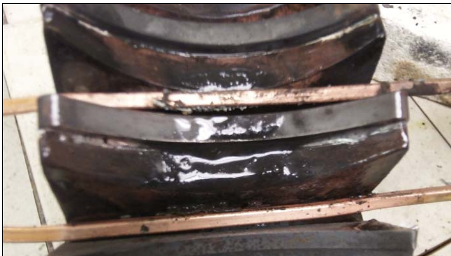
The assembly inside the induction heating coil after brazing
