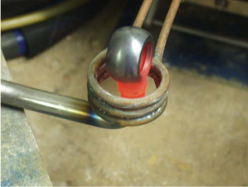
Brazing the steel tube and fitting assembly together
