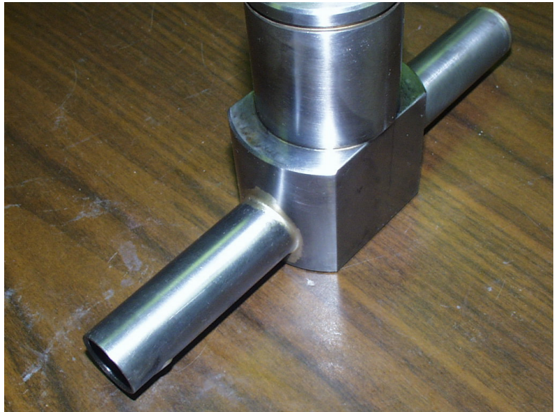
Completed assembly with both joints brazed
