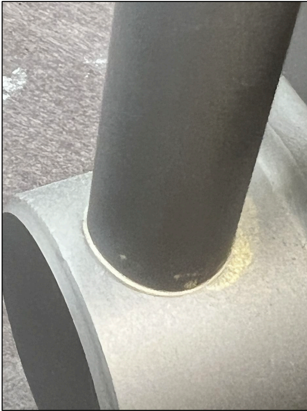
The assembly after brazing.
