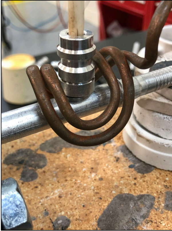
The assembly in the induction pancake coil.
