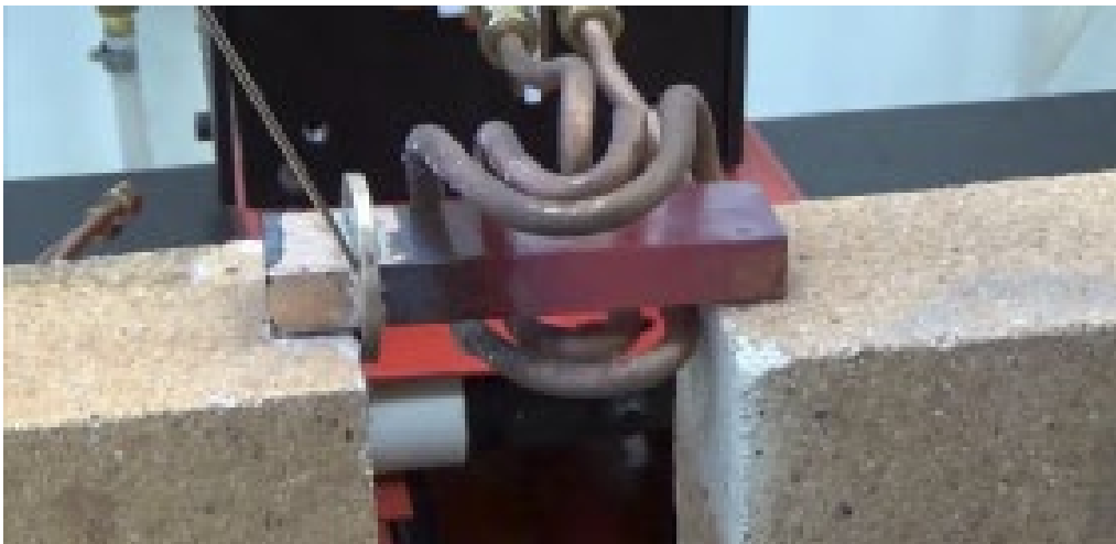
Small brass fitting being brazed to the copper tube.
