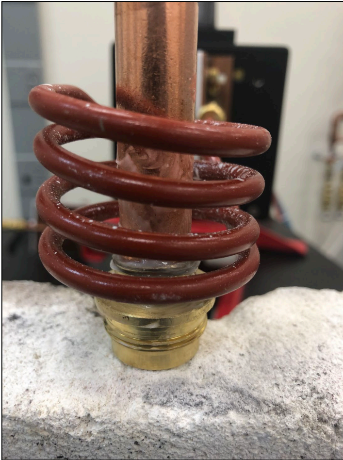
The copper and brass assembly inside the coil.
