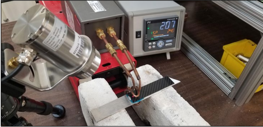
The assembly being heated inside the u-shaped induction coil.
