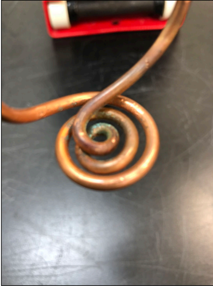
The pancake coil heating the wire sample.
