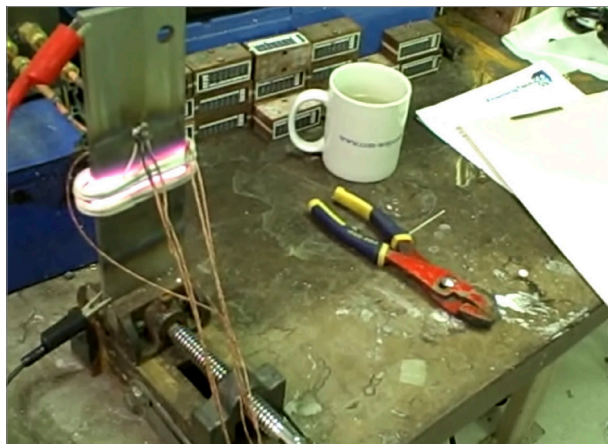
The Hanes nickel alloy block inside the specially designed coil.
