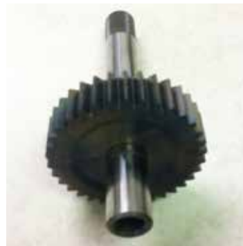
The gear and shaft after shrink fitting.
