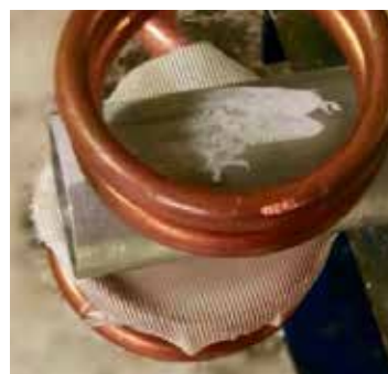
The split helical coil enabled easy loading.
