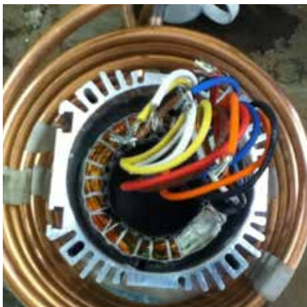
The aluminum motor housing and stator after shrink fitting inside the induction heating coil.
