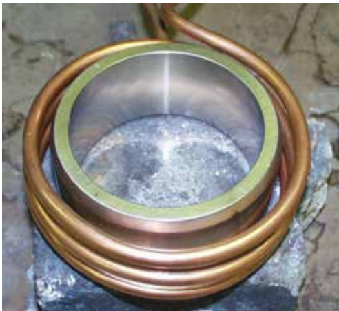
Stainless steel sleeve heating in coil prior to shrink fit application.
