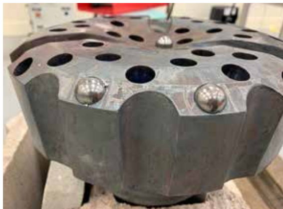
The drill head with carbide bits.
