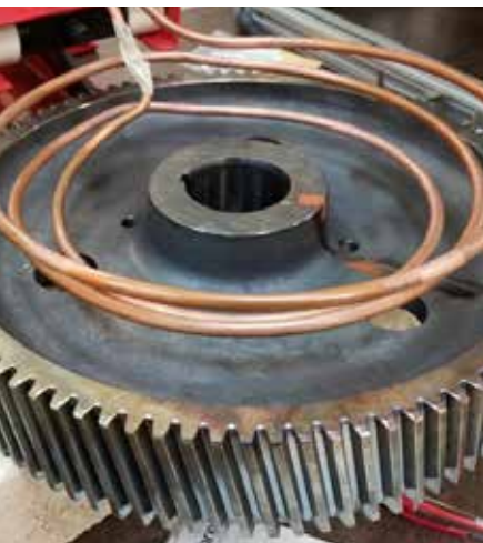
The induction setup with the gear and coil.
