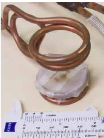
The split helical coil enabled easy loading.
