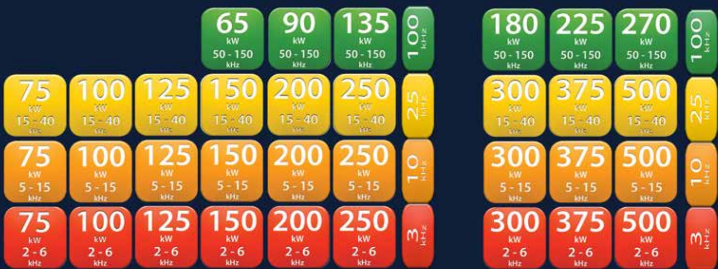
65 to 250 kW with models covering the four frequency bands 50 to 150 kHz 15 to 40 kHz 5 to 15 kHz 2 to 6 kHz
