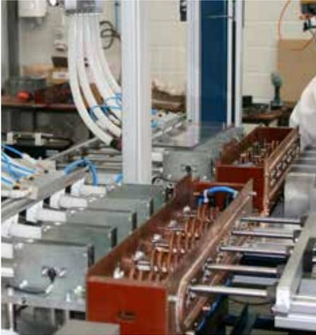
**Induction annealing systems allow ammunition manufacturers to eliminate excessive part handling and inventory, thus producing less scrap and achieving a higher yield for less cost.**
